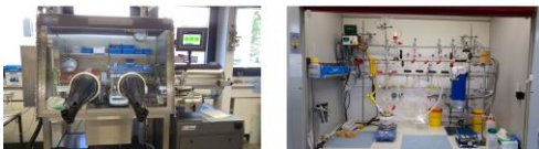
Perovskite NCs (top) are synthesized by an organic method involving the use of a glovebox (bottom left) and a Schlenk line (bottom right).
